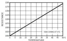
Fig. 3. Pt1000 Temperature vs. resistance
