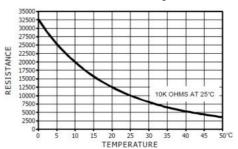
Fig. 1 NTC10K Temperature vs. resistance
