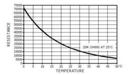
Fig. 2 NTC20K Temperature vs. resistance
