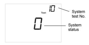
Press and hold  $\triangle$  and  $\overline{V}$  buttons 3 seconds to enter test mode.
