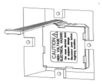
Step 3 Place Back cover over junction box, insert and tighten mounting screws.
