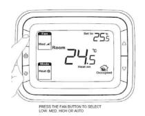
Fan can be selected as manual or automatic 3-speed operation. In Manual mode, the fan is switched to the selected speed via control output Gh, Gm, Gl. In automatic mode, fan speed depends on the difference between room temperature and setpoint. When room temperature reaches setpoint, valve will be closed and meanwhile, fan will be closed either.
