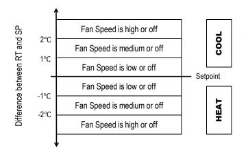
Fig. 1. Fan Speed Ramping Control Algorithm
