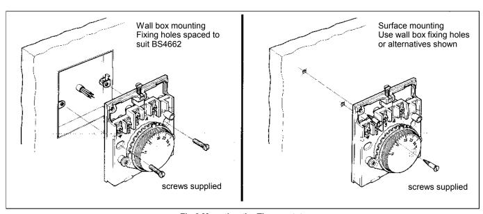
Fig.2 Mounting the Thermostat
