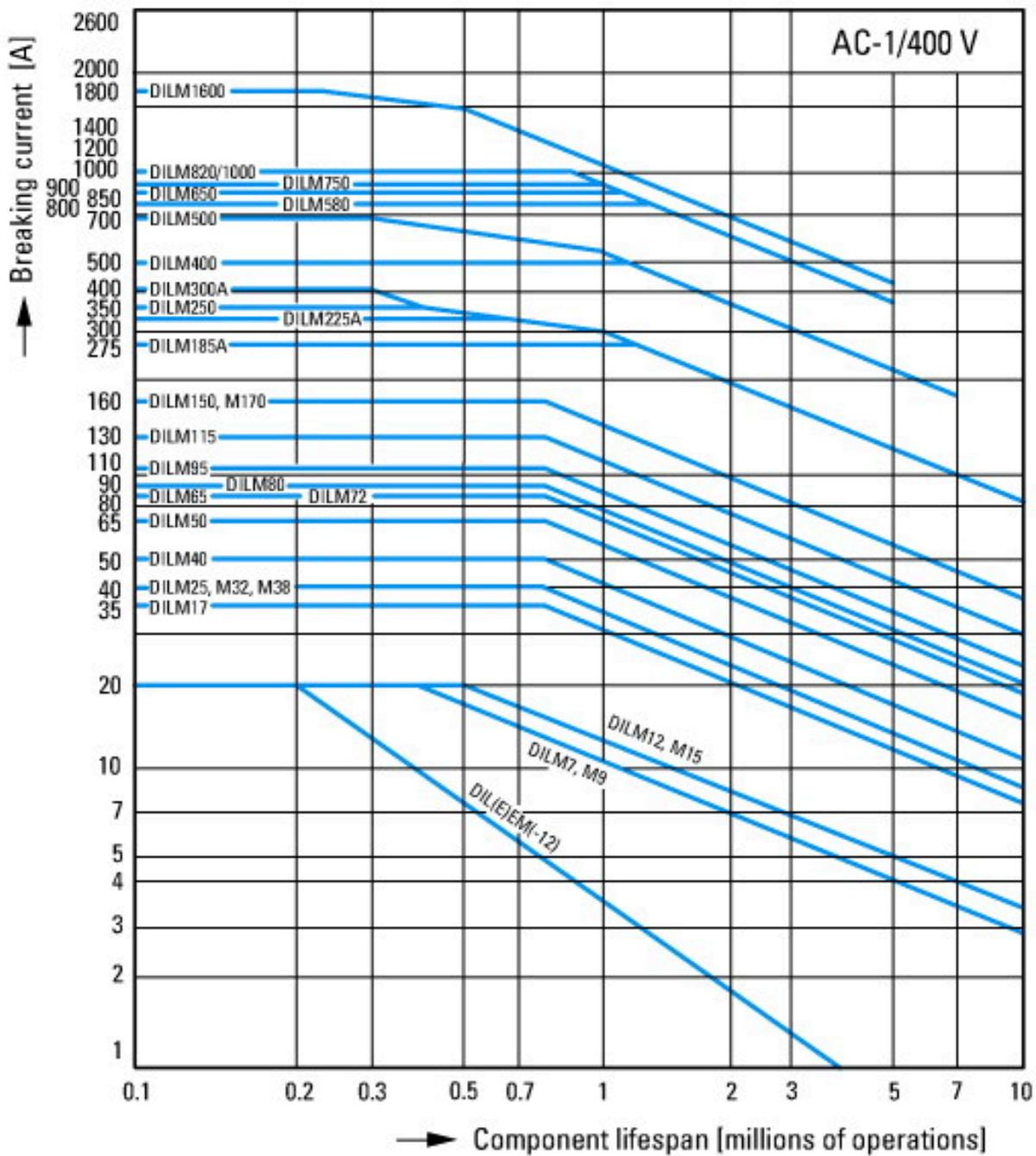
Switching duty for non-motor loads, 3-pole, 4-pole
