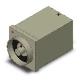
24 VAC 50/60 Hz, 24 VDC, Output Time-limit: DPDT, Power OFF-delay, Time range: 0.05 to 0.6 min (4 range), 8-pin
